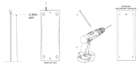
Insert wall plugs into drilled holes. Use hammer to fit wall plugs into position. Insert screws provided into wall plugs and screw into position, leaving 5mm to hang the HyGenikx unit.
